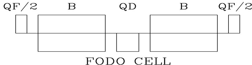
$$\begin{aligned} \mathbf{M} &= \begin{pmatrix} 1 & 0 \\ -\frac{1}{2f} & 1 \end{pmatrix} \begin{pmatrix} 1 & L_1 \\ 0 & 1 \end{pmatrix} \begin{pmatrix} 1 & 0 \\ \frac{1}{f} & 1 \end{pmatrix} \begin{pmatrix} 1 & L_1 \\ 0 & 1 \end{pmatrix} \begin{pmatrix} 1 & 0 \\ -\frac{1}{2f} & 1 \end{pmatrix} \\ &= \begin{pmatrix} 1 - \frac{L_1^2}{2f^2} & 2L_1(1 + \frac{L_1}{2f}) \\ -\frac{L_1}{2f^2}(1 - \frac{L_1}{2f}) & 1 - \frac{L_1^2}{2f^2} \end{pmatrix} \end{aligned}$$
