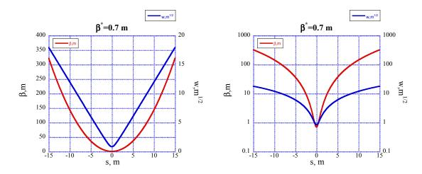
Plot of beta-function and beam envelope in 30-m long straight section with  $\beta$ \*=0.7 m – typical for RHIC interection region.
