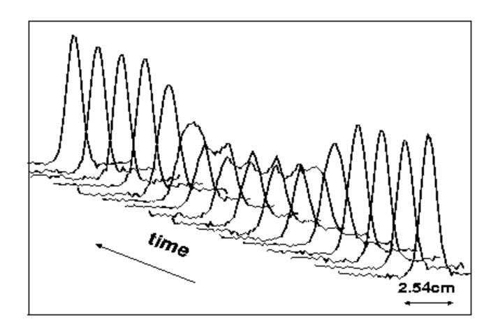
The beam profile measured from an ionization profile monitor (IPM) at the AGS during the adiabatic turn-on/off of an rf dipole. The beam profile appeared to be much larger during the time that the rf dipole was on because the profile was an integration of many coherent synchrotron oscillations. After the rf dipole was adiabatically turned off, the beam profile restored back to its original shape (Graph courtesy of M. Bai at BNL).
