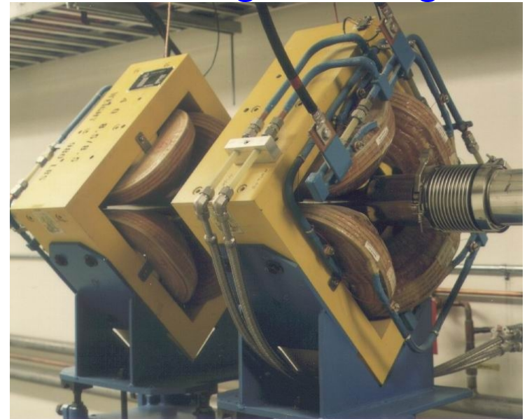
Quadrupole: strong focusing
