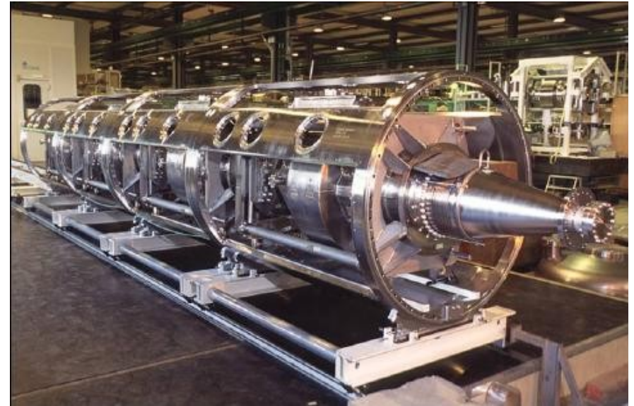
LHC RF cavity string - 7 TeV ring
