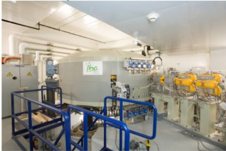
Figure 2. IBA 230 MeV resistive cyclotron for proton therapy
