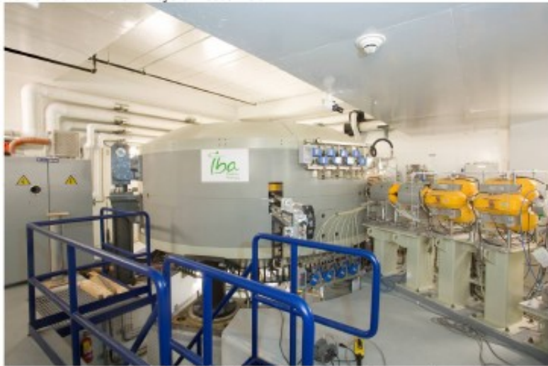
Figure 2. IBA 230 MeV resistive cyclotron for proton therapy
