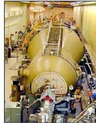
One of the two (face-to-face) stages of the 15 MV Tandem-Van de Graaff at BNL. Can accelerate 40 different types of ions.
