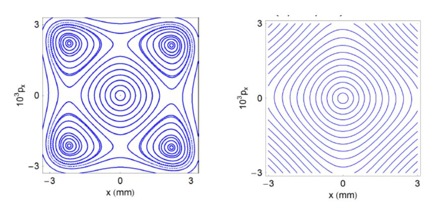
Example of  $\{x,Px\}$  phase-space diagram showing trace of the particles motion in accelerators: a set of particles with initial coordinate were seeded n the plot and then traced for a large number of turns. Stable motion results in periodic and semi-periodic results in "orbits – semi-closed trajectories" in the phase space.
