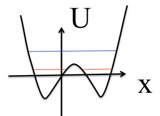
While for high energies (blue) trajectory is unique, for lower energies (red) there are two distantly separated areas of the motion.
