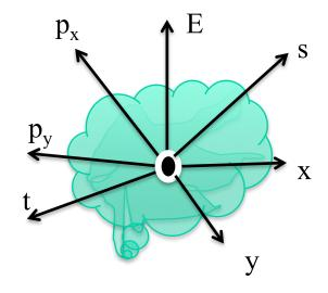
The full set of coordinates and momenta of particle (or a ensemble of particles)  $\{q_i, P_i\}$  is called phase space. Naturally dimension of the phase space is always even: 2,4,6.., 2n. While motion in the coordinate space  $\{q_i\}$  can be rather arbitrary, the same motion in the phase space satisfies a number of very strong constrains, e.g. there is a number of invariants.
