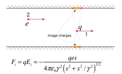
$$F_{x} = q\left(E_{x} - c\beta B_{y}\right) = \frac{qex}{4\pi\varepsilon_{0}\gamma^{4}\left(s^{2} + x^{2}/\gamma^{2}\right)^{3/2}}$$
