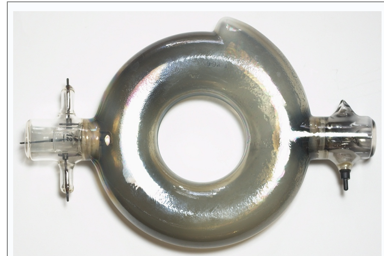
SVETLANA RBK6-6E Betatron 6 MeV. Manufacturing date around 1991. In-situ radiotherapy and radiographic non destructive testing: containers, ship hulls, weapons [Ref.: http://lampes-et-tubes.info/xr/xr033.php?l=d ]
