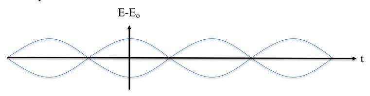
• When synchronous particles gaining or losing energy, topology of the phase space changes: particles can cross from the upper part to the bottom part (typical for qn acceleration or a energy loss case) or from the bottom to top (for a deceleration case) – these particles will be lost by hitting energy acceptance of the lattice
