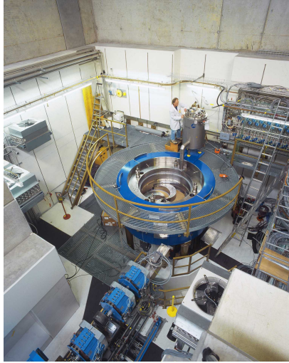
Fig. 1.3 Superconducting-coil isochronous spiral-sector AVF cyclotron at PSI, providing 250 MeV, 500 nA beams for hadrontherapy.
