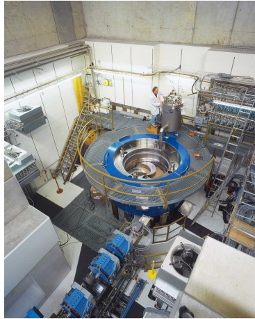
Fig. 1.1 Superconducting-coil isochronous spiral-sector AVF cyclotron at PSI, providing 250 MeV, 500 nA beams for hadrontherapy.
