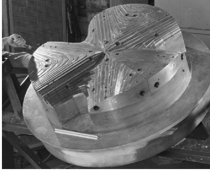
Fig. 1.13 Azimuthal pole shaping in Thomas-style AVF cyclotron.
