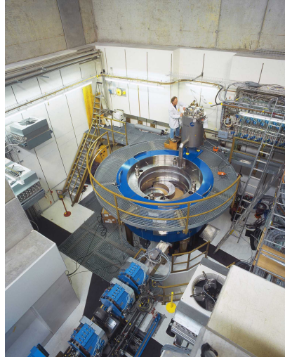
Fig. 1.3 Superconducting-coil isochronous spiral-sector AVF cyclotron at PSI, providing 250 MeV, 500 nA beams for hadrontherapy.
