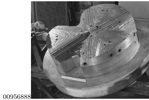
Fig. 1.13 Azimuthal pole shaping in Thomas-style AVF cyclotron.
