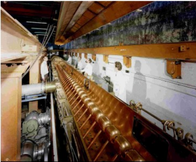
202M Hz/70 MeV Alvarez injector linac at ISIS, RAL.
