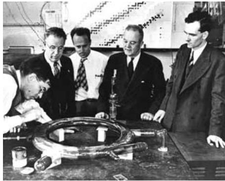
Vacuum chamber of GE synchrotron
