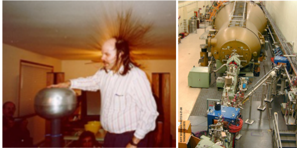
Fig. 2.5. Does not matter how much fun is electrostatic and how many good electrostatic “dinosaurs” are in basements of our universities, Maxwell equation prohibits multiple acceleration is DC electric field:
