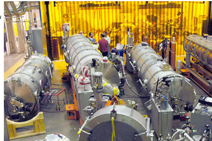
Fig. 2.11. CEBAF, a 12 GeV (was operating at 6 GeV) recirculating SRF linac at Thomas Jefferson Accelerator Facility. On the right – SRF accelerating modules. Upgrade to be finished by 2015.
