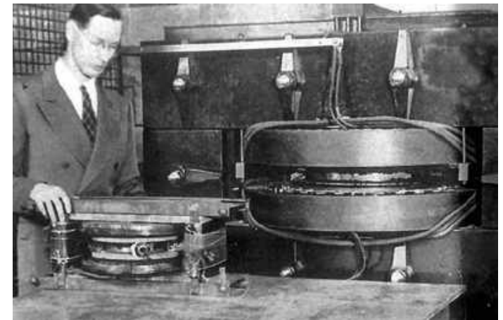
Schematic of circular betatron (left) and Kerst with his induction (betatron) accelerator (right)
