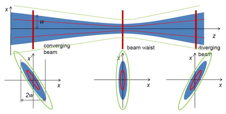
Along a beamline the orientation and aspect ratio of the beam ellipse in x, x' changes, but area (emittance) remains constant.
