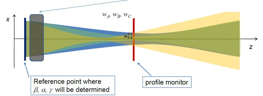
$$w^{2} = c^{2} \beta \varepsilon - 2 c s \alpha \varepsilon + s^{2} \gamma \varepsilon, \quad \begin{pmatrix} c & s \\ c' & s' \end{pmatrix} = \begin{pmatrix} 1 & L \\ 0 & 1 \end{pmatrix} \cdot \begin{pmatrix} m_{11}(I_{mag}) & m_{12}(I_{mag}) \\ m_{21}(I_{mag}) & m_{22}(I_{mag}) \end{pmatrix}$$
