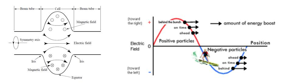
The RF field must be synchronous (correct phase relation) with the beam for a sustained energy transfer.
