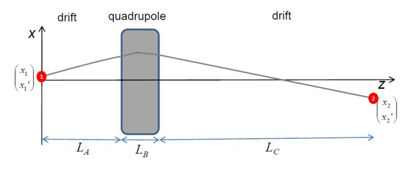
$$M_{\textit{Drift}} = \begin{pmatrix} 1 & L \\ 0 & 1 \end{pmatrix} \qquad M_{\textit{Quadrupole}} = \begin{pmatrix} \cos(\sqrt{k}L) & 1/\sqrt{k}\sin(\sqrt{k}L) \\ -\sqrt{k}\sin(\sqrt{k}L) & \cos(\sqrt{k}L) \end{pmatrix}$$
