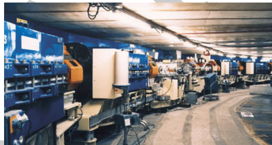
Fig. 10.4 SATURNE II strong focusing 3 GeV synchrotron at Saclay, successor in the late 1970s of Saturne I weak focusing synchrotron (Fig. 9.1). It was the first strong focusing synchrotron to accelerate polarized ion beams
