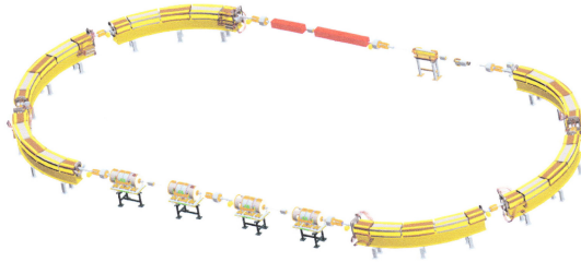
Fig. 10.5 The ion rapid cycling medical synchrotron (iRCMS) [6], an RCS aimed at providing ion beams for the treatment of cancer tumors
