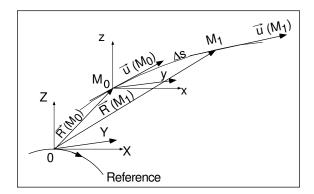
Fig. 1.4 Position vector  $\mathbf{R}$  and normalized velocity vector ( $\mathbf{u} = \mathbf{v}/v$ ) of a particle in zgoubi frame. A  $\Delta s$  push takes the particle from position  $M_0$  to position  $M_1$
