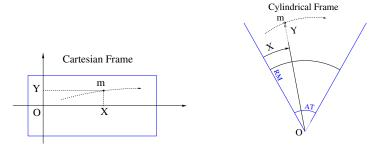
Fig. 1.5 Cartesian and cylindrical reference frames in optical elements
