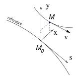
**Fig. 1.2** Moving frame  $(M_0; s, x, y)$  along a reference line.  $M_0$ , at path distance s from some origin, is the projection of particle location M(x, y, s) on the reference
